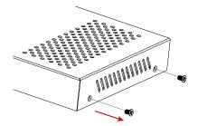
Attach the installation bracket to the enclosure using the screws provided. The bracket is attached to the enclosure as shown.
